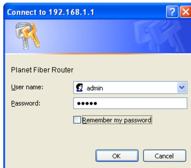
If the user name and password are correct, you will login Fiber Router successfully and see the status page. Now you can configure the Fiber Router for your needs.
