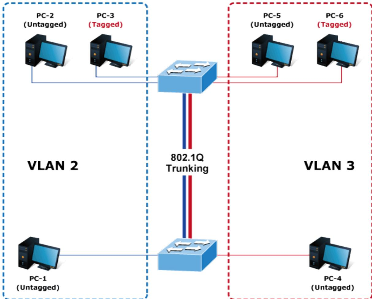
Figure 4-3-53: VLAN Trunking between two 802.1Q aware switches
