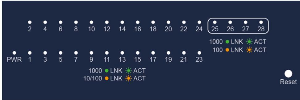
Figure 2-1-25: GS-4210-24T4S(R) LED Panel
