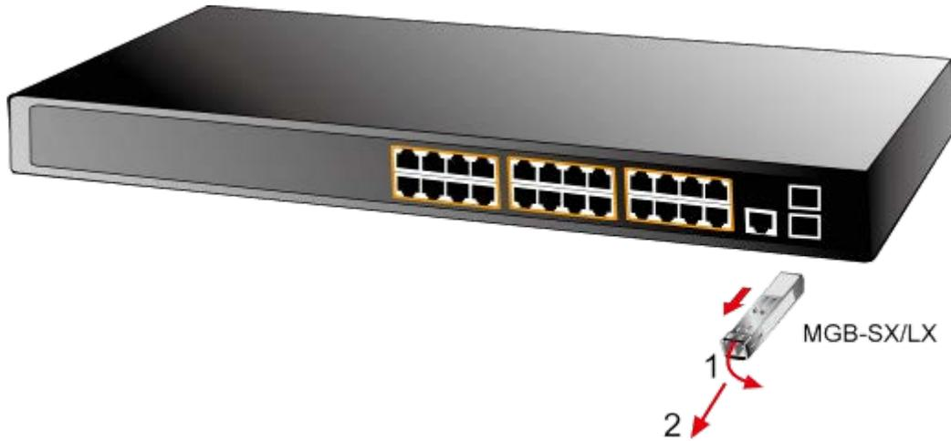
**Figure 2-1-45:** How to Pull Out the SFP Transceiver
