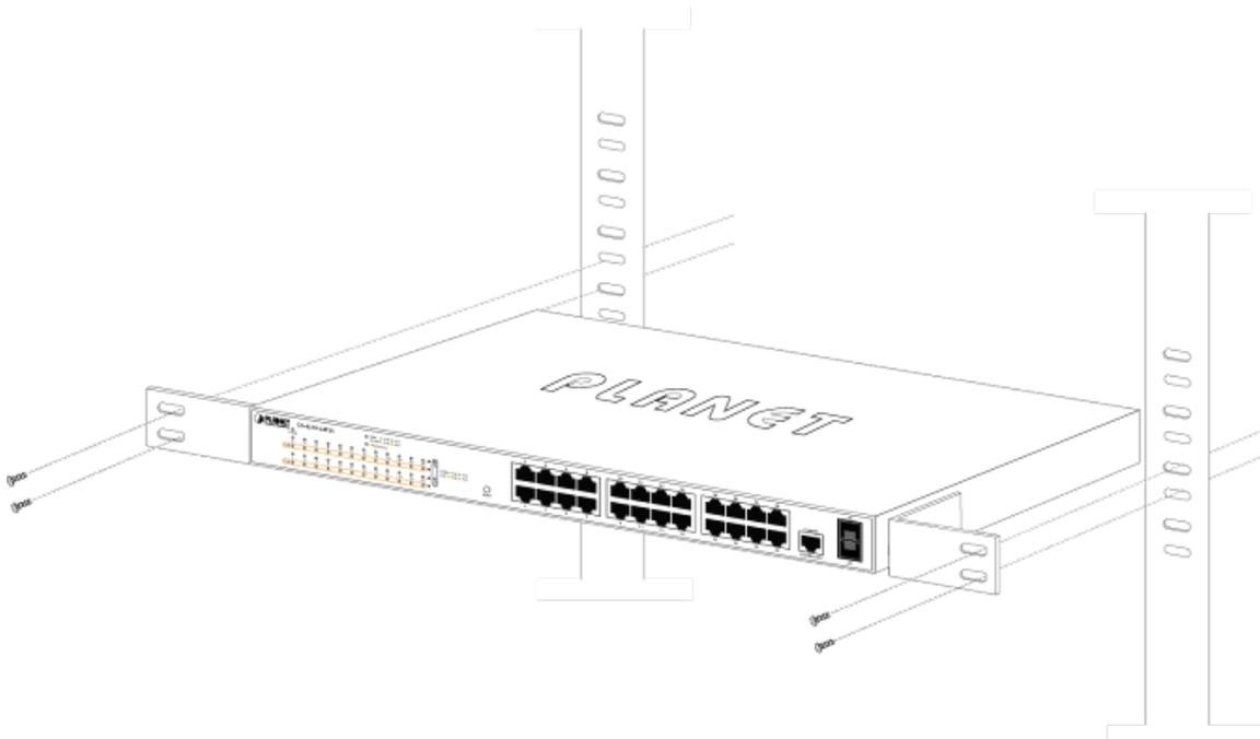
**Figure 2-1-43:** Mounting Managed Switch in a Rack
