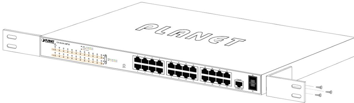
**Figure 2-1-42:** Attach Brackets to the Managed Switch
