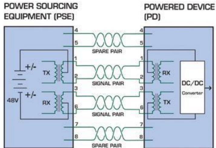
Figure 8-2: Power Supplied over the Data Pins
