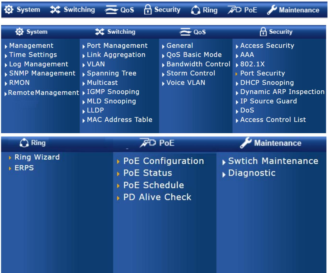
Figure 4-1-5: Managed Switch Main Functions Menu
