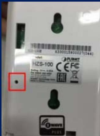
j. HZS-200: Press the program button of the HZS-200 for 3 times within 3 seconds to be included.
