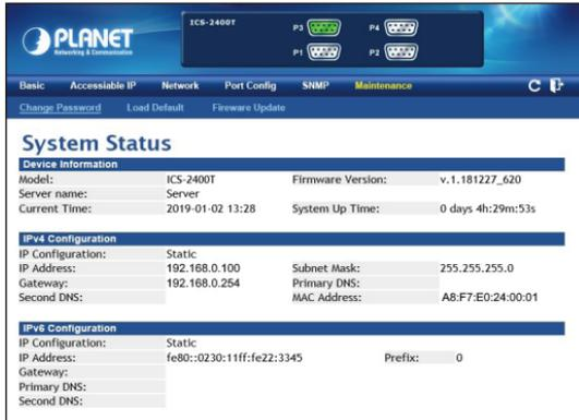
**Figure 4-3:** Web Main Screen of Industrial Serial Server
