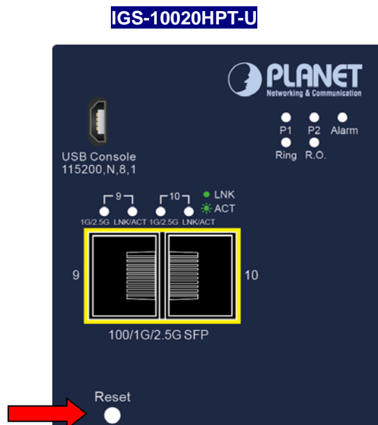
Figure 2-2: 10020HPT-U Reset Button
