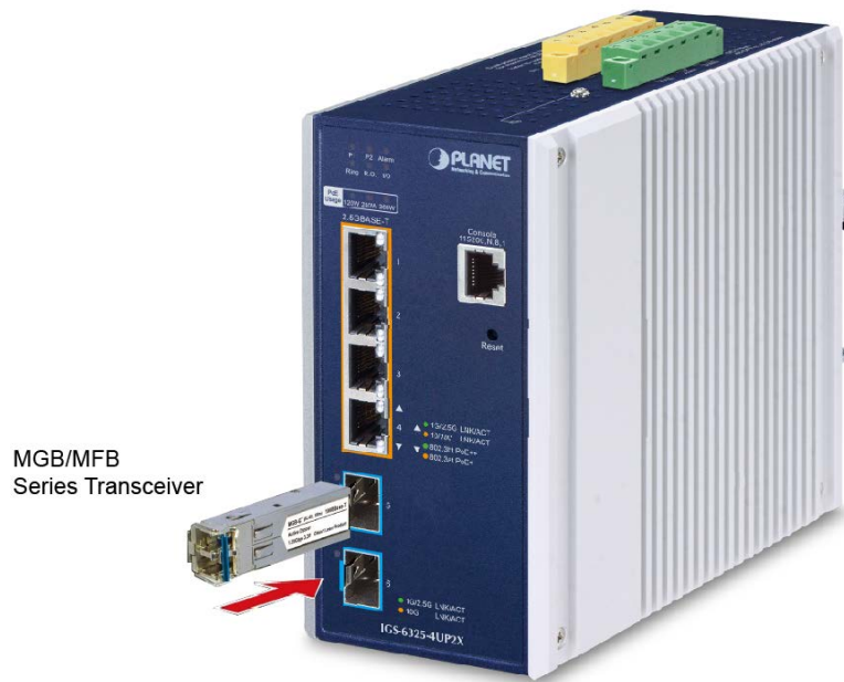
Figure 2-8 : Plugging in the SFP Transceiver
