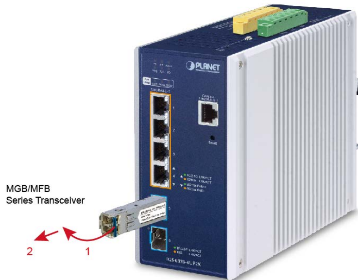
Figure 2-9: Pulling out the SFP Transceiver Module
