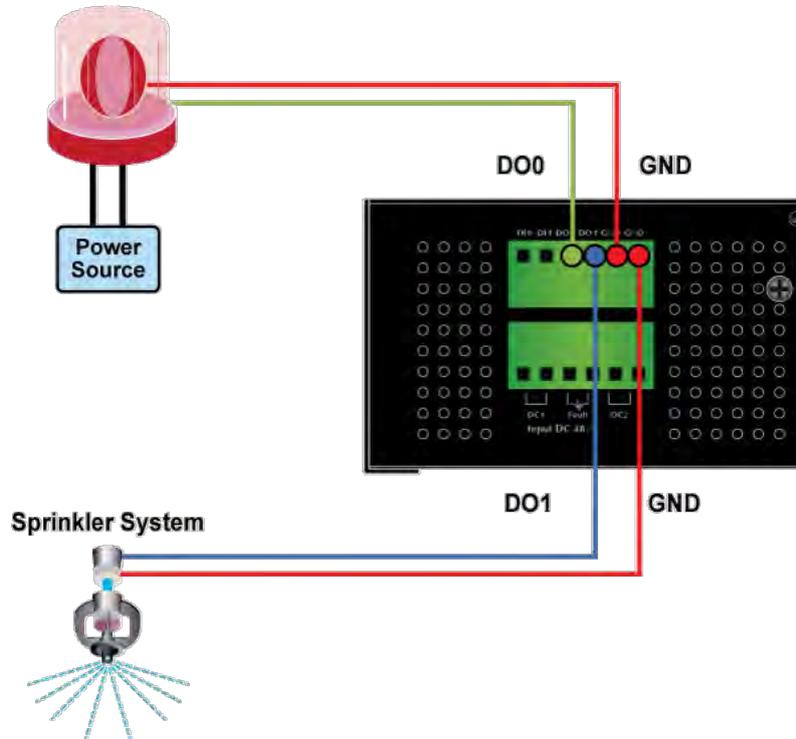
**Figure 2-16:** Wiring DO0 and DO1 to Open Detector
