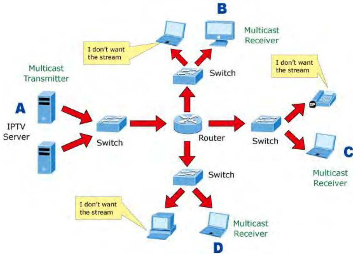
Figure 4-3-5-2: Multicast Flooding
