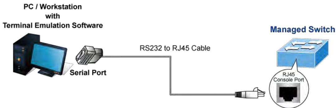
Figure 3-1: Industrial L2+ Managed Switch Console Connectivity
