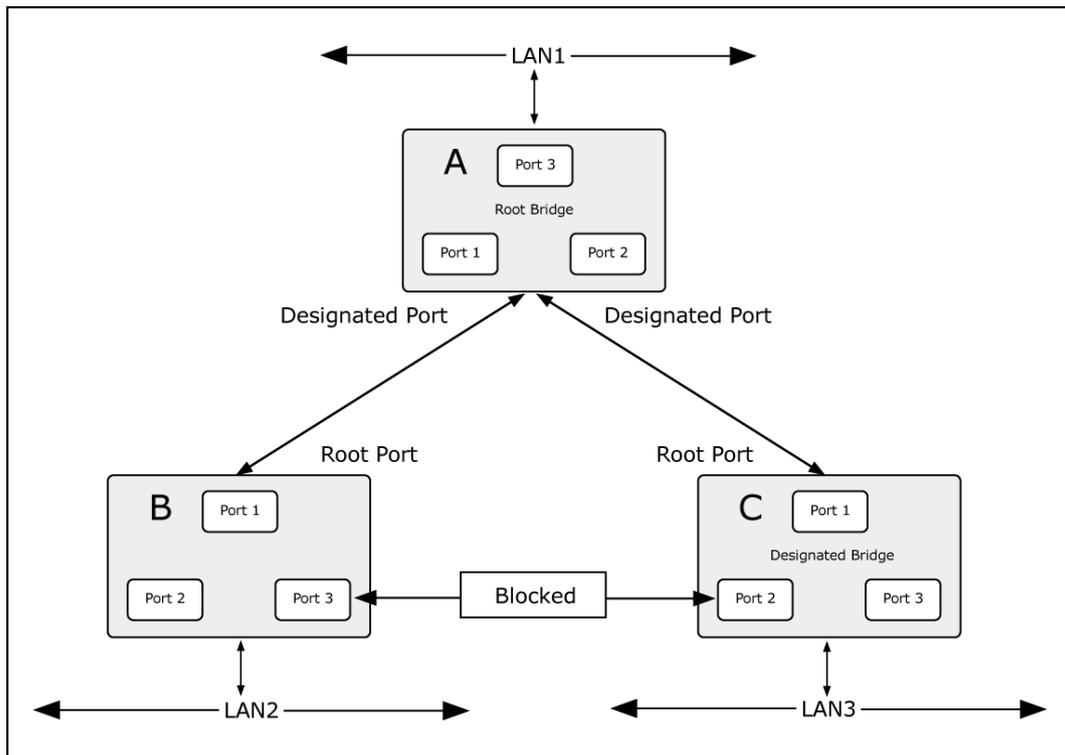
**Figure 4-3-4-3: After Applying the STA Rules**
