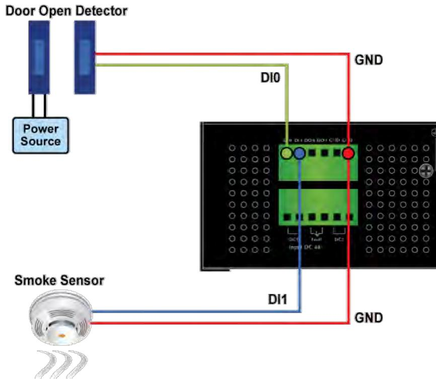
**Figure 2-15:** Wiring DI0 and DI1 to Open Detector
