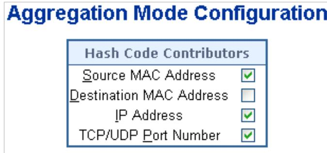
Figure 4-3-2-2 : Aggregation Mode Configuration Page Screenshot
