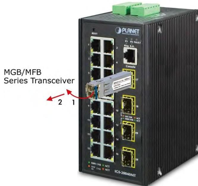
**Figure 2-18:** Pulling out the SFP/SFP+ Transceiver Module
