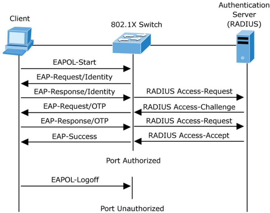
Figure 4-5-2-2: EAP Message Exchange
