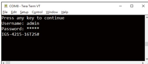
**Figure 4-1:** Industrial Managed Switch Console Login Screen
