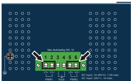
Figure 3-1: IGS-4215-16T2S Inlet Power Socket
