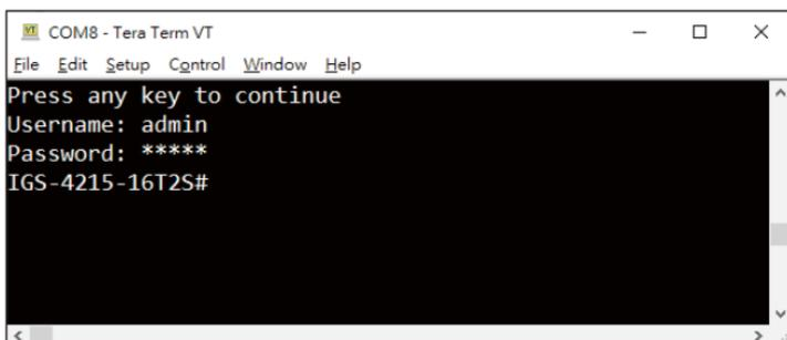
**Figure 4-2:** Industrial Managed Switch Console Login Screen
