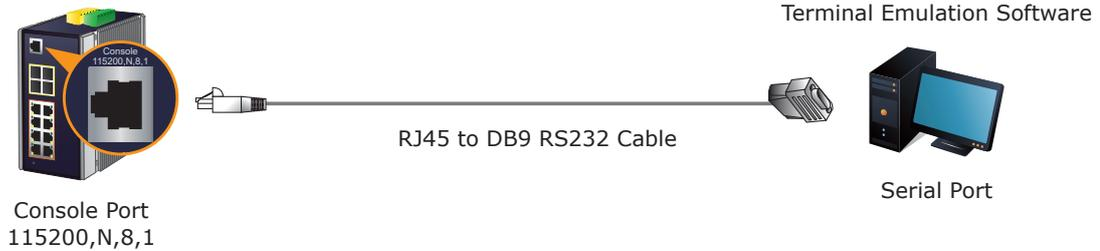
A terminal program is required to make the software connected to the IGS-5225 series Industrial Managed Switch.
