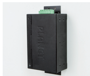
Side Wall Mounting (Space saving)
