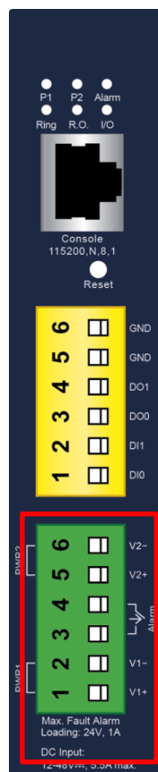
Figure 2-1-4: IMS-6325-5 DC Power Connector
