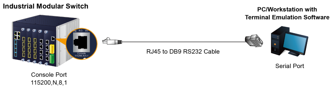
Figure 3-3-1: RJ45-to-DB9 console connection
