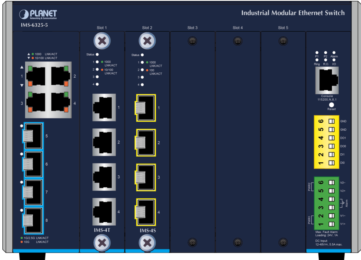
Figure 2-1-1: IMS-6325-5 Switch Front Panel
