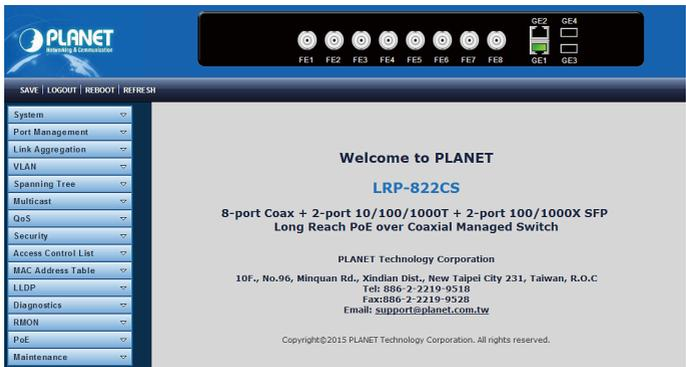
**Figure 7-3:** Web Main Screen of LRP Managed Switch
