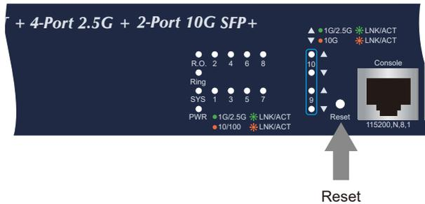
Figure 5-1: MGS-6320 Series Reset Button
