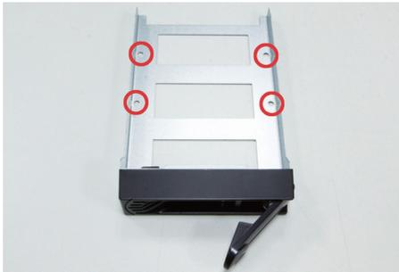
7. Once the HDD is placed in the tray, flip it over and secure the HDD with the screws.
