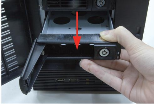
3. Place the HDD on the bottom of the tray.
