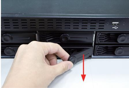
5. Pull out the HDD tray further to be removed.
