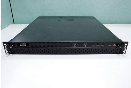
2. To remove the front plate, turn the tool-less screws on both sides counter-clockwise to loosen it from the unit. Please note the screws will still be attached to the front plate even after the screws are completely loosened from the unit.
