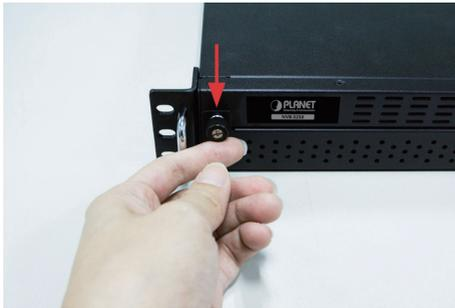
3. Simply pull to remove the front plate once the screws are loosened from the unit.
