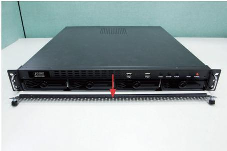
4. Pull out the HDD tray by the latch.
