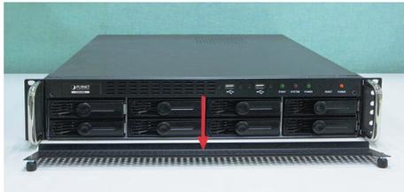
4. Pull out the HDD tray by the latch.
