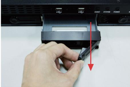
6. Once the tray is removed from the unit, note there are four holes, which are used to secure the HDD.
