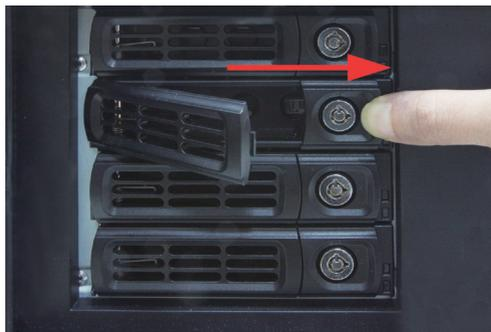
2. Pull the HDD tray out of the case.
