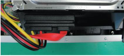
7. Fix HDD brackets on system with screws.
