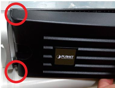
2. Press the latch and push the right end towards the unit's right handle until it clicks into place.
