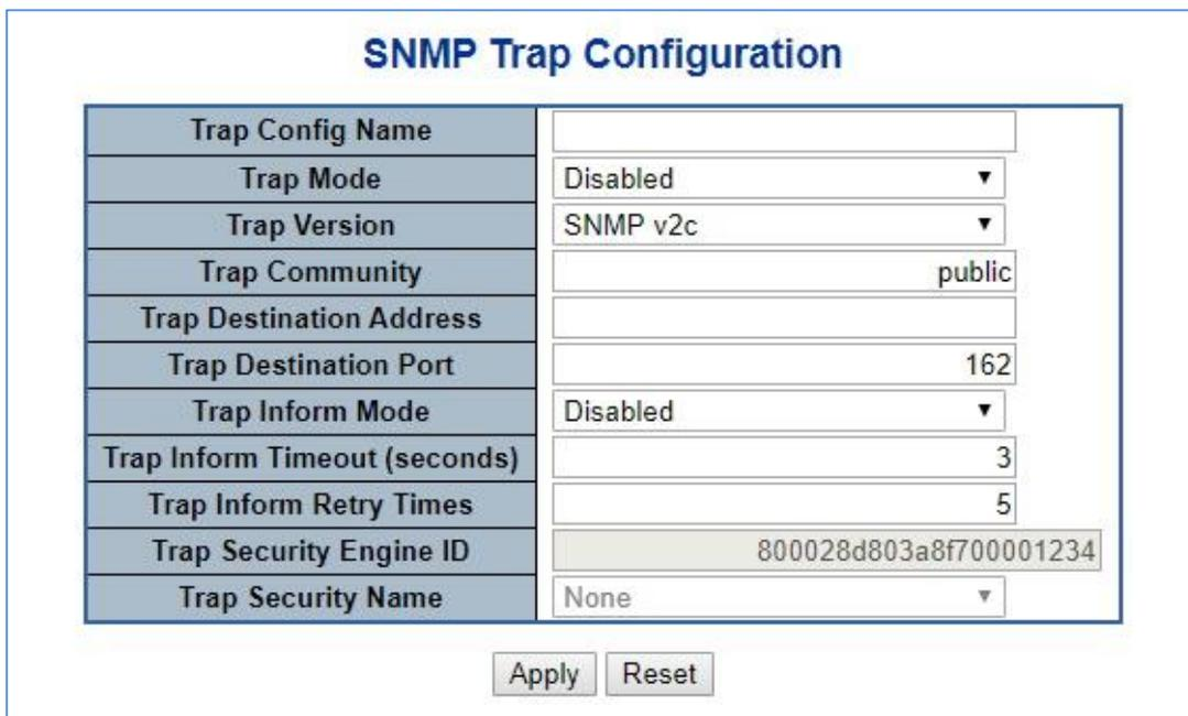
Figure 4-2-24: SNMP Trap Configuration Page Screenshot
