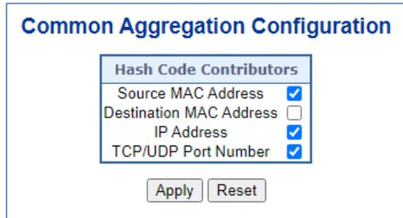
**Figure 4-3-12:** Common Aggregation Configuration Page Screenshot
