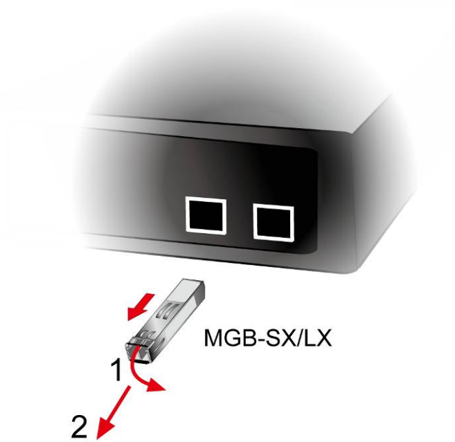
Figure: How to Pull Out the SFP/SFP+ Transceiver
