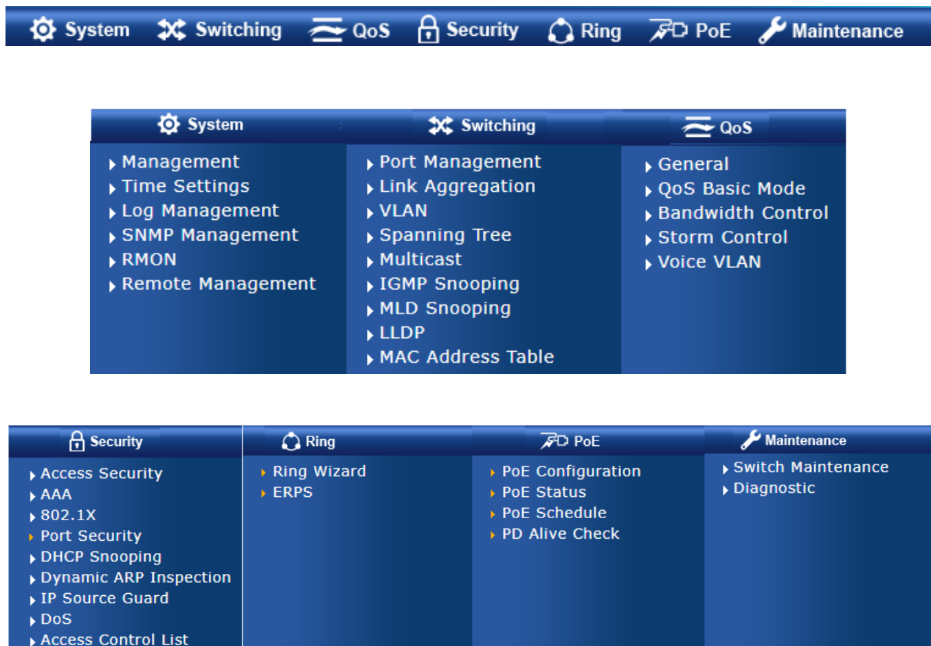
Figure 4-1-2 Managed Switch Main Functions Menu
