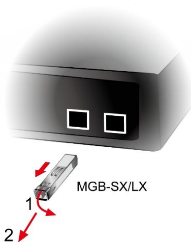
Figure 2-1-8 How to Pull Out the SFP Transceiver
