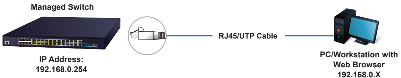
Figure 5-1: IP Management Diagram
