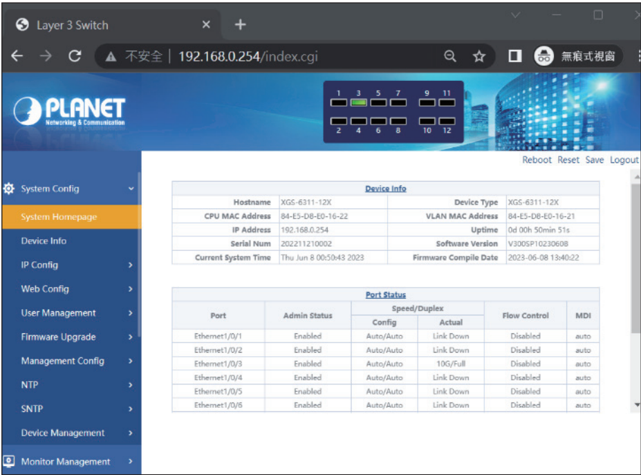
Figure 5-5: Web Main Screen of Managed Switch
