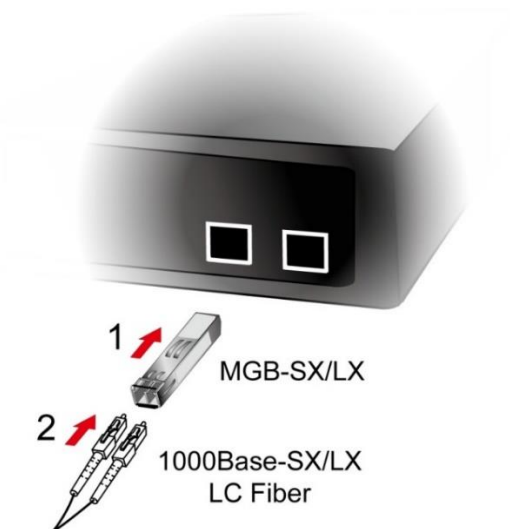
Figure 2-2.3 Plug in the SFP transceiver
